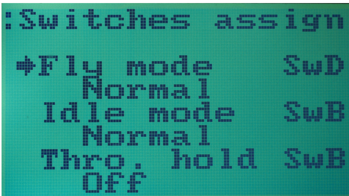
Photo 3B Assigning Switch D whilst in Fly Mode to “Normal” & “Sport”
